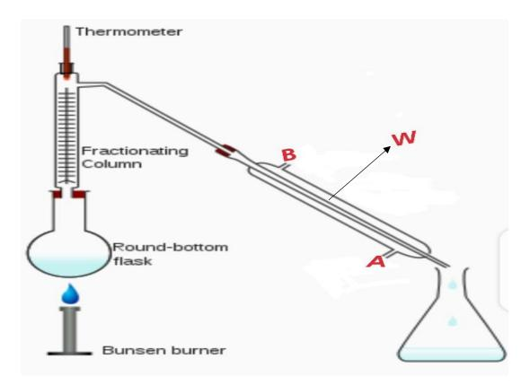
(i) Name the piece of apparatus labelled W
