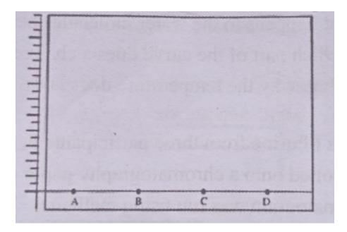
After development **A**, **B**, and **C** were found to have moved 8cm, 3cm and 6cm respectively. **D** had separated into two spots which had moved 6cm and 8cm
